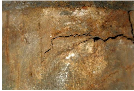
Figure 0.2: Image showing stress corrosion cracking ( https://us.sfs.com/learn-more/detect-prevent-hydrogen-assisted-stress-corrosion-cracking )
