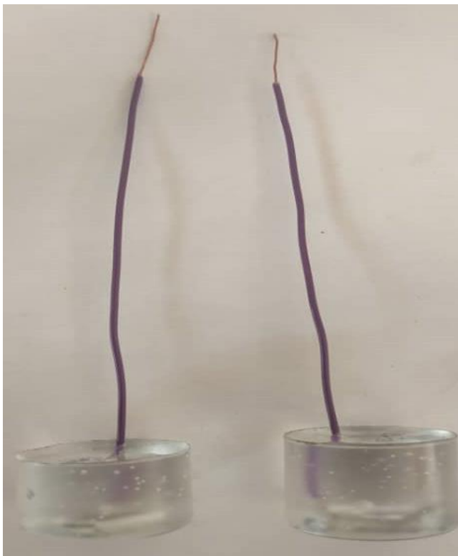
Figure 0.4: Cold mounted polished metal specimens ready to be used for electrochemical experiments.
