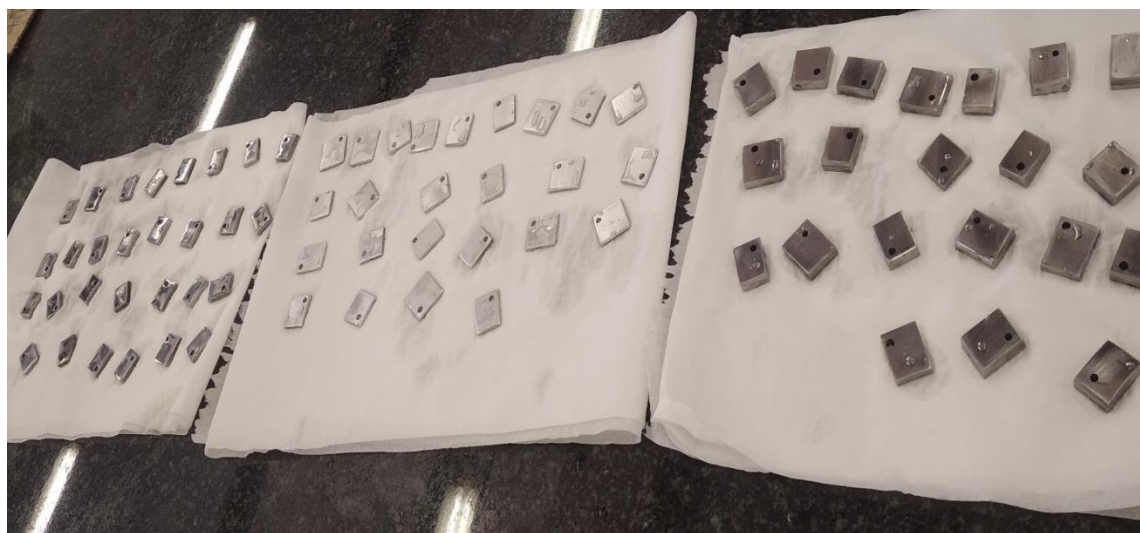
Figure 0.3: Weight loss metal specimens after drilling and grinding before polishing.
