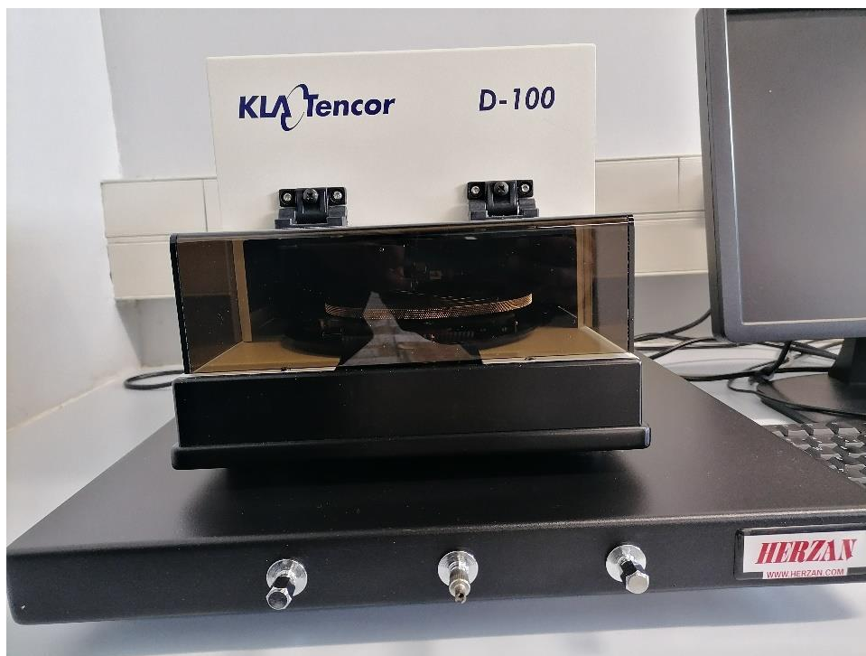
Figure 11: KLA Tencor D-100 Surface Profiler.
