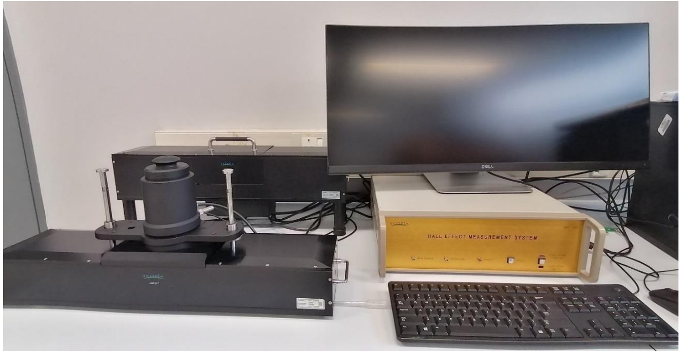
Figure 18: The ECOPIA HMS5500 Hall Effect Measurement System.
