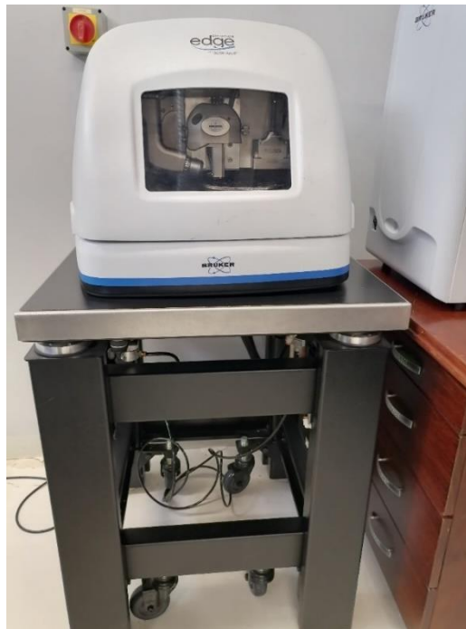
Figure 15: The BRUKER Atomic Force Microscope.
