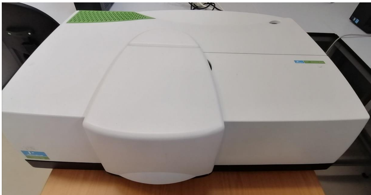
Figure 17: The Perkin Elmer 750 UV/VIS/NIR Spectrophotometer.
