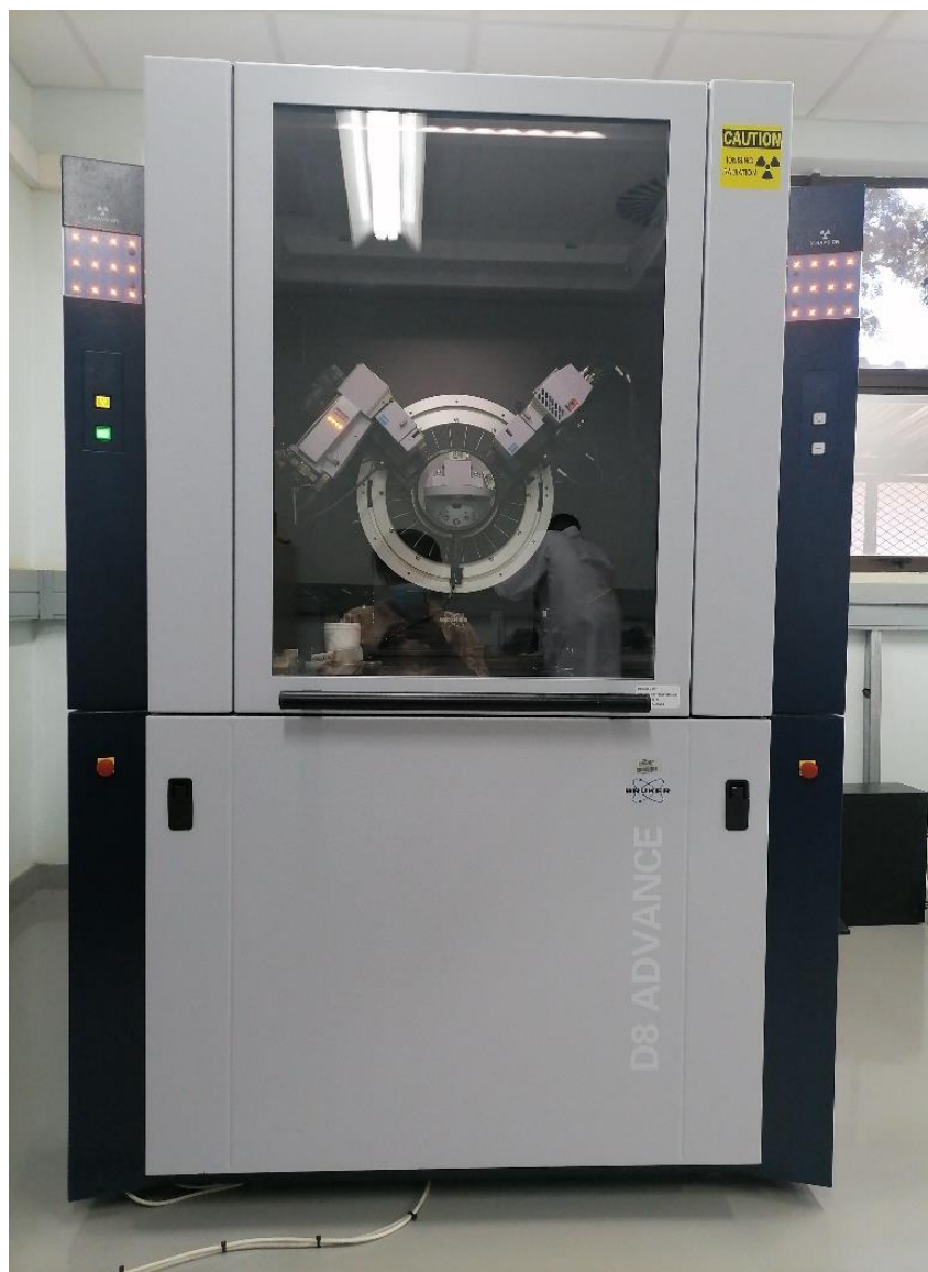
Figure 12: Bruker D8 Advanced X-ray diffractometer.
