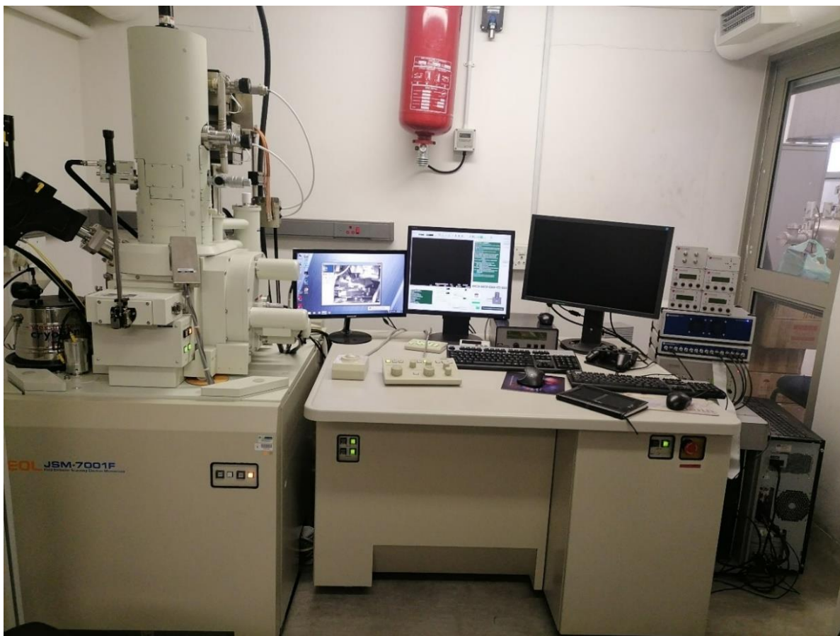
Figure 16: JEOL JSM-7001F Field Emission Scanning Electron Microscope.
