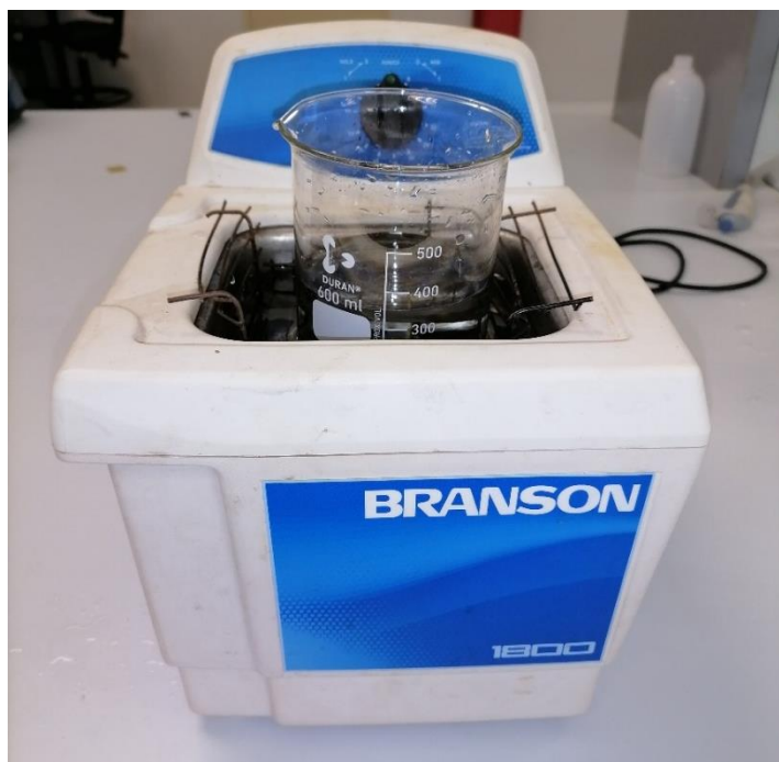
Figure 6: The ultrasonic tank used to clean the glass substrates
