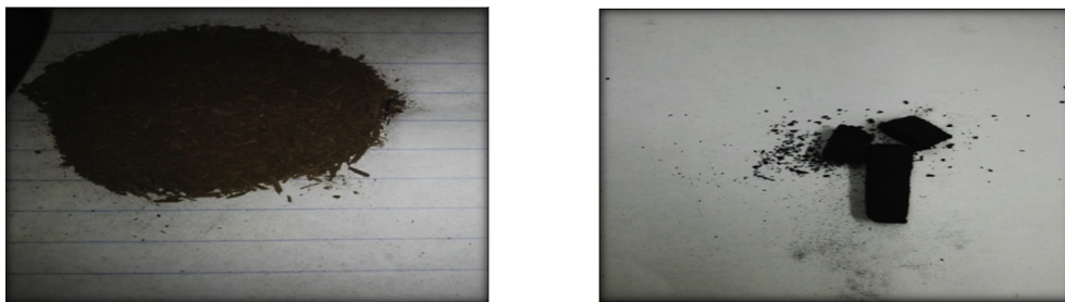
Fig. 7 – Change in colour of biomass before (left) and after (right) torrefaction.
