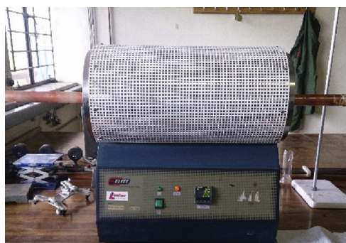
Fig. 3 – Laboratory tube furnace used for torrefaction.
