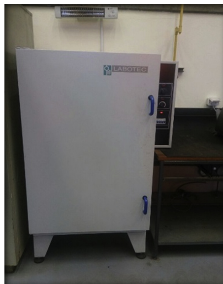
Fig. 2 – Oven for drying biomass samples from Labotec.
