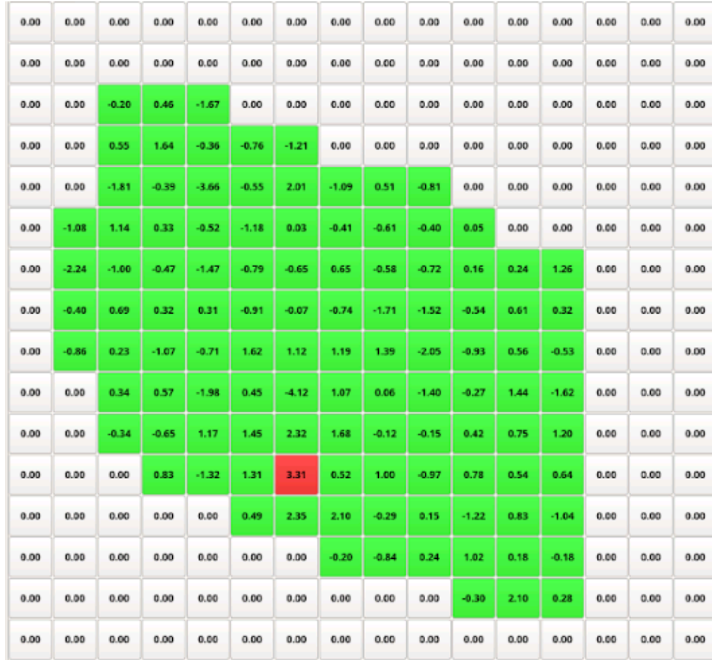
Figure 4.8: User interface showing a 30 mm Kimberlite with a 12 mm imitator. The green colour shows the region occupied by the kimberlite ore, the grey colour shows an empty space of the tray while the red colour shows the region occupied by the diamond imitator.
