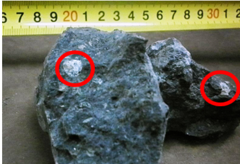
Figure 5.9: Two diamond inclusions detected at the Mir mine using the tagged neutron method.
