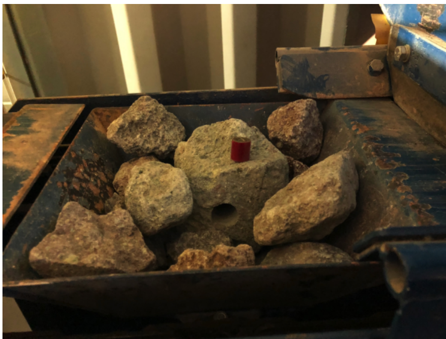
Figure 5.2: Ore arrangement in a tray. A hole is drilled in a kimberlite ore and a diamond imitator inserted in the hole.
