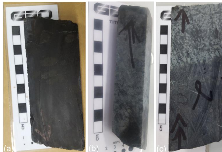
Figure 2.5. Photographs of rock types of the massive harzburgite (a) unit with minor pyroxenite (b) and feldspathic pyroxenite (c) to the ultramafic sequence in MF38. The sharp contact between harzburgite and feldspathic pyroxenite is shown in (c).
