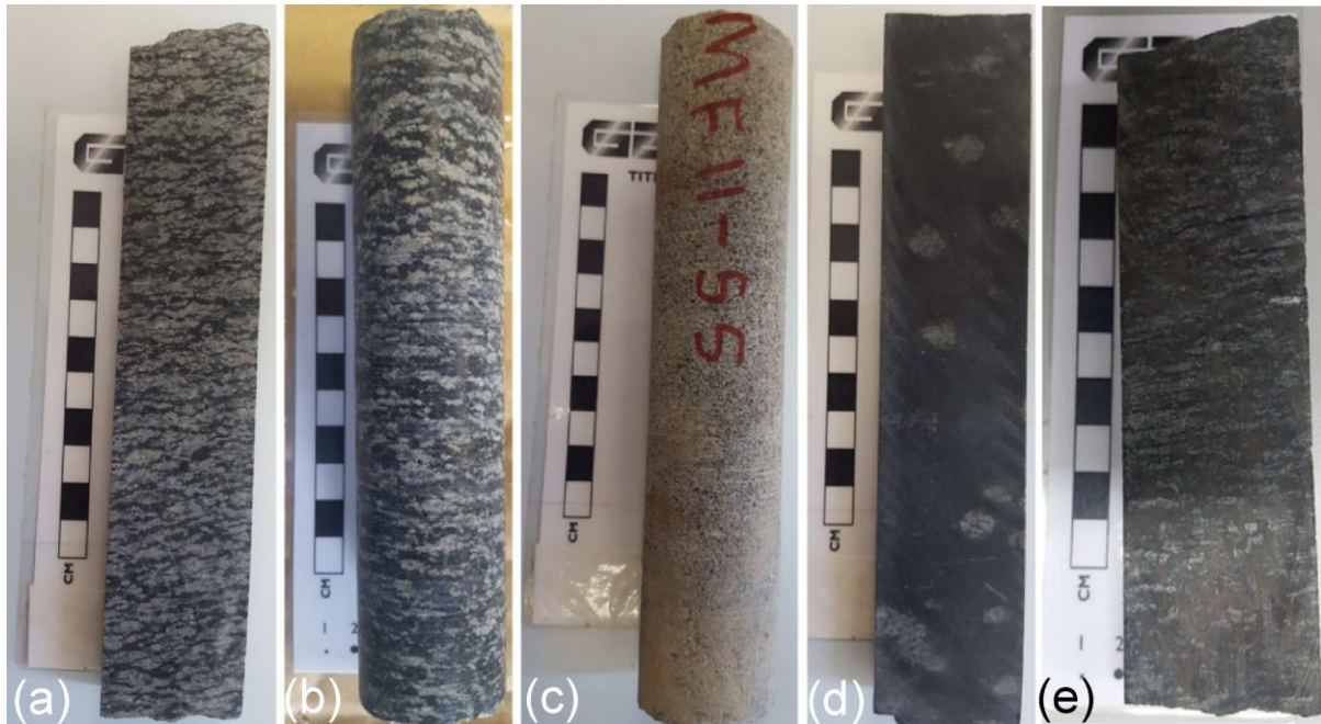
Figure 2.7. Photographs illustrating rock types of the basal pyroxenite with minor norite unit to the ultramafic sequence in MF11. (a), (b) feldspathic pyroxenite; (c) melanorite; (d) massive pyroxenite. Feldspathic pyroxenite from a similar pyroxenite unit above in the stratigraphy is shown in (e) .
