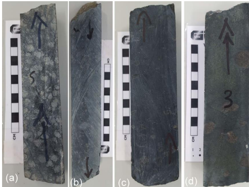
Figure 2.4. Photographs of rock types from the dominant pyroxenite (a, b) with minor harzburgite (c) and dunite (d) unit of the the cumulate textured ultramafic sequence in MF38. Unlike the typical cumulate textured occurrence (a), a medium-grained pyroxenite variant (b) occurs in this unit.
