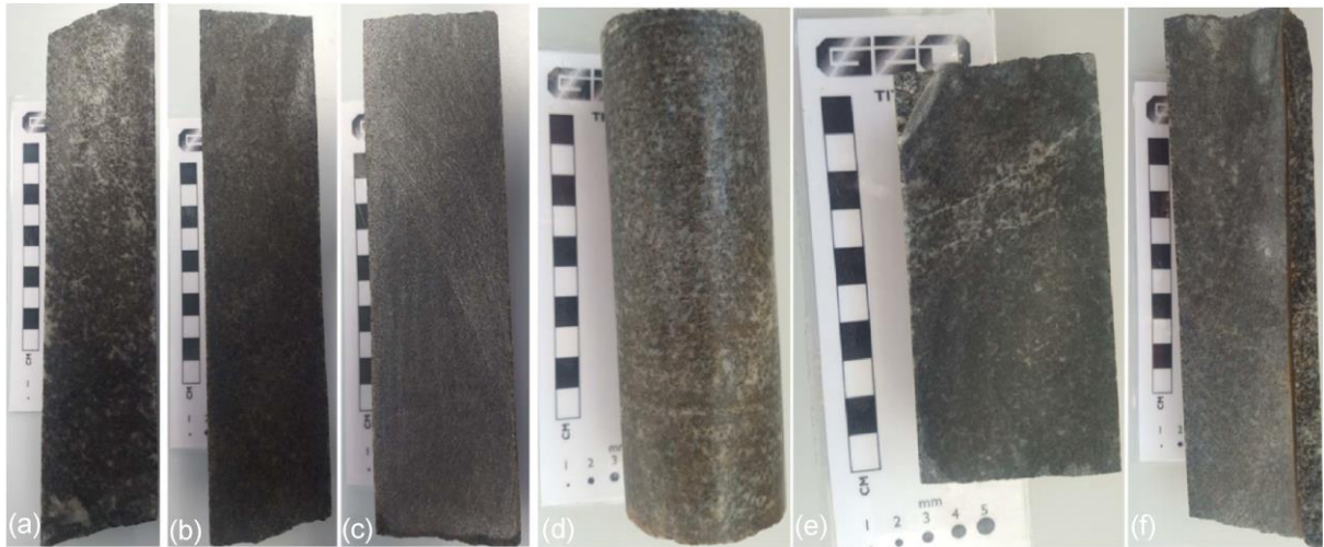
Figure 2.10. Photographs illustrating rock types of the basal gabbronorite unit with feldspathic pyroxenite from the mafic sequence in MF9. (a), (b), (e), (f) melanocratic gabbronorite; (c) leucocratic gabbronorite; (d) feldspathic pyroxenite.
