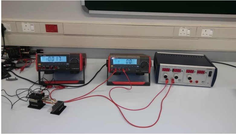
Figure 3.10: Picture of the Four-point probe setup consisting of the power supply, voltmeter, ammeter and connecting wires.
