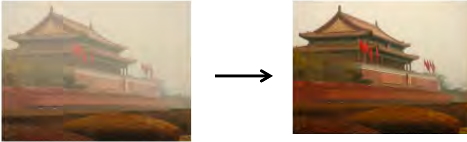
Figure 2.5: Results of DCP image dehazing using weighted guided image filter by Li et al.,( 2015)
