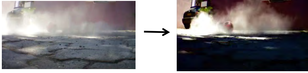
Figure 5.4: Images before and after thick fog removal using the DCP
