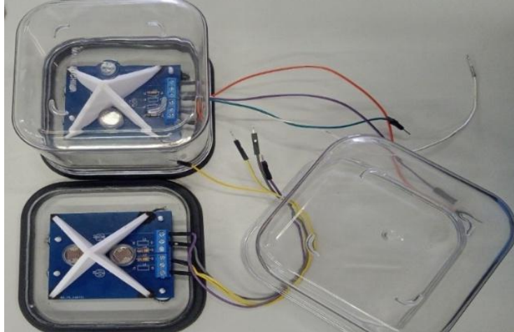
Figure 3-30. Sensor array housing and circuit board.
