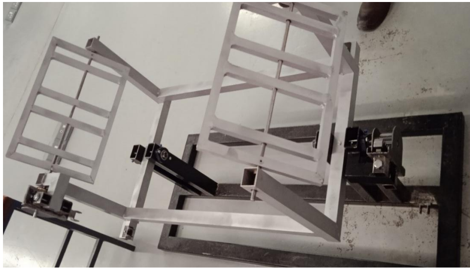
Figure 3-29. Fabricated dual axis solar tracking framework.
