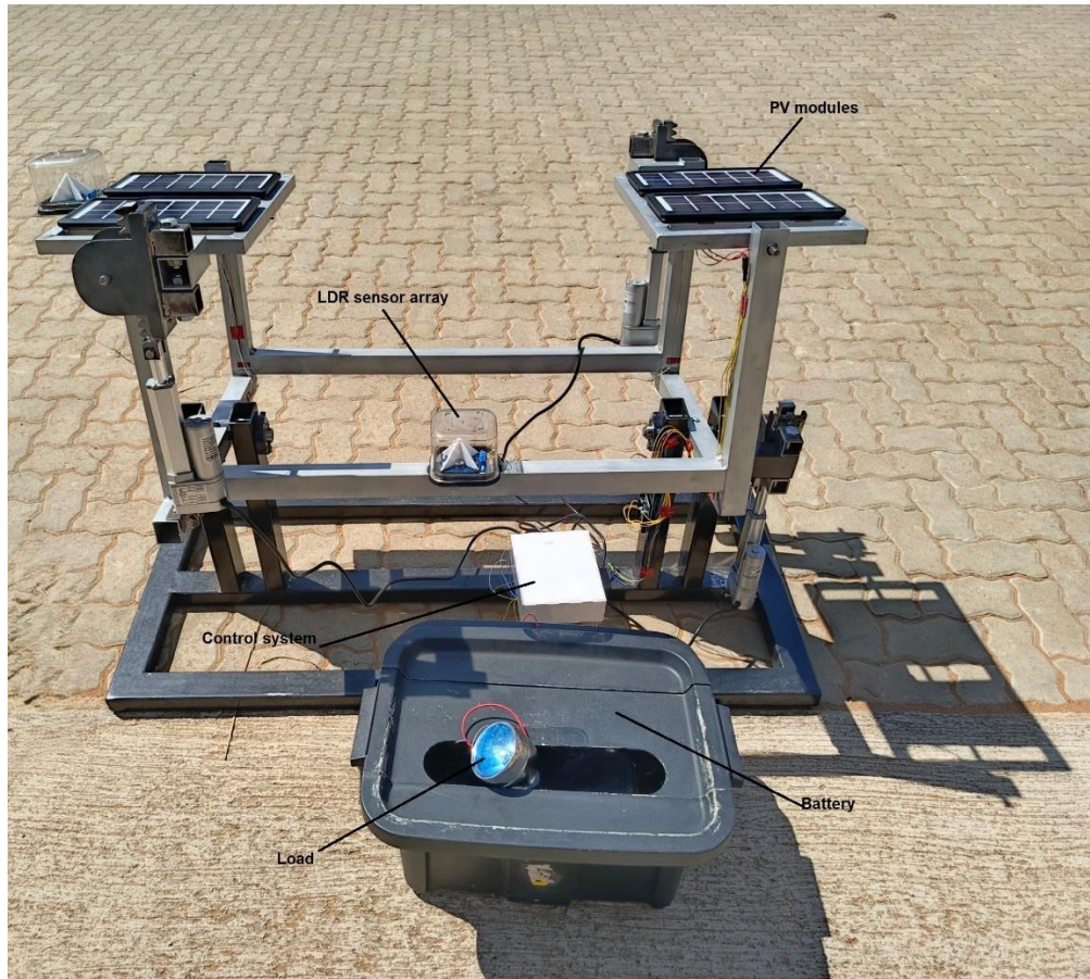
Figure 4-25. Prototype of a two-axis solar tracker.
