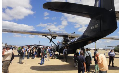
Figure 9. PBX-6A is an amphibious aircraft that uses parasol wing [Picture taken by the first author].
