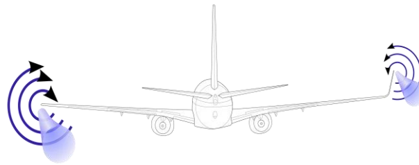
Figure 16. Wingtip vortices formation on a wing with and without a winglet.
