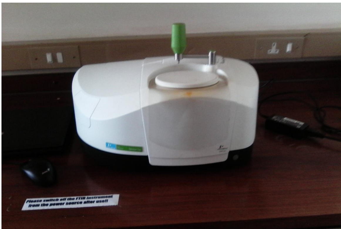
Figure 3.6: A picture of the Perkin Elmer Spectrum Two ATR-FTIR spectrophotometer equipment used
