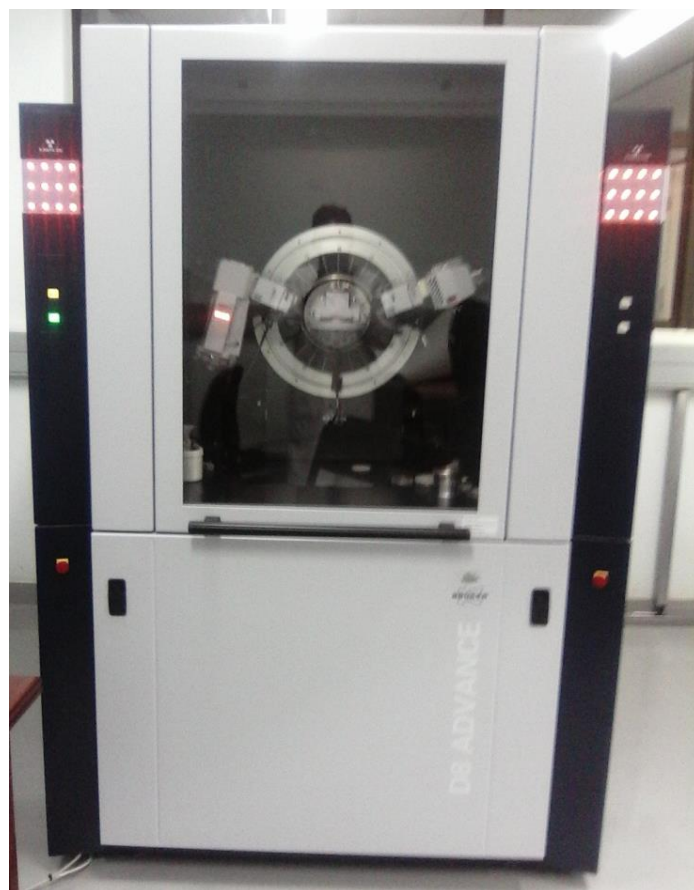
Figure 3.4: A picture of the Bruker D8 Advance XRD equipment used
