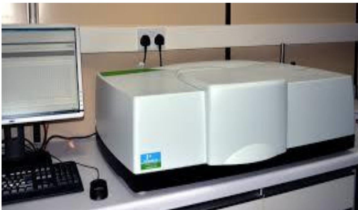
Figure 3.7: A picture of the Lambda 750 Perkin Elmer UV-Vis-NIR spectrophotometer used
