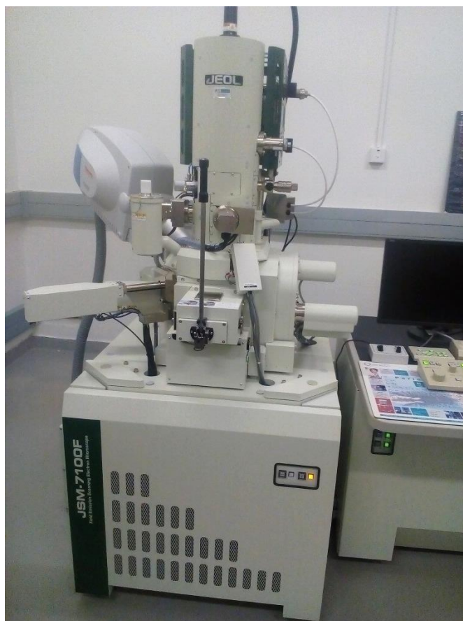
Figure 3.5: A picture of the JEOL JSM 7100F FESEM equipment used in this study
