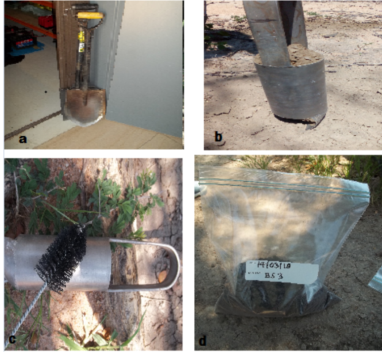
Figure 3.3: Equipment used in soil sampling a) a shovel used for ground clearing b) an auger for collecting soil from 15 cm deep c) brush for cleaning the auger and d) a polyethylene plastic bag to contain soil samples.
