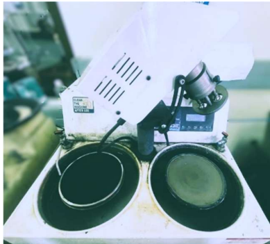
Figure 3.6: Qualitest Qualipol-VTD-SA machine used for grinding and polishing.
