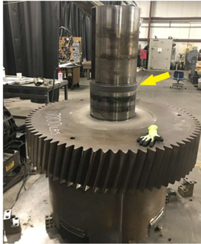
Plate 5.1: Laser refurbished bearing surface on bull gear (Swinson, 2020).
