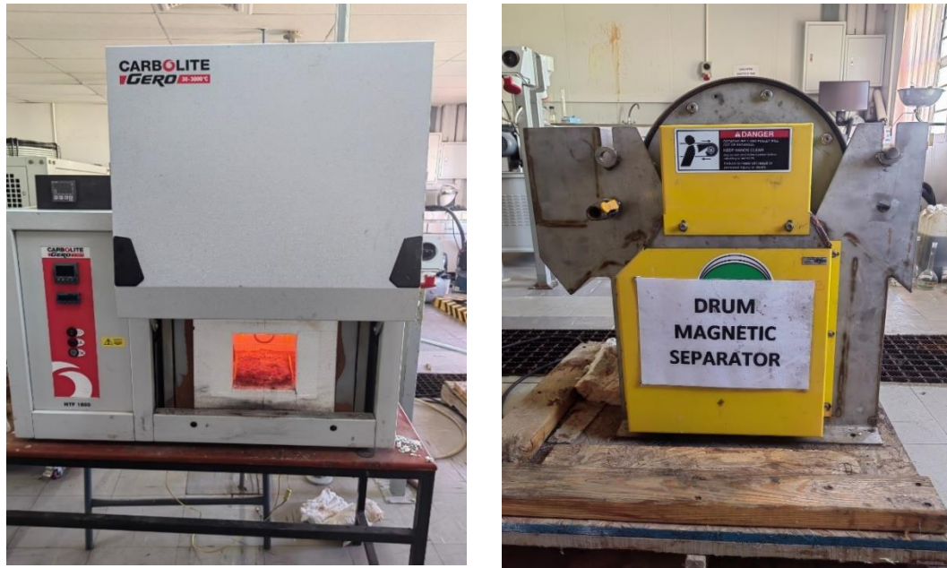
Figure 16. Equipment used in the beneficiation process; a) Carbolite Gero furnace; b) Drum magnetic separator
