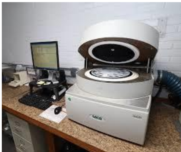
Figure 13. Thermogravimetric analyser (TGA 701) used for proximate analysis
