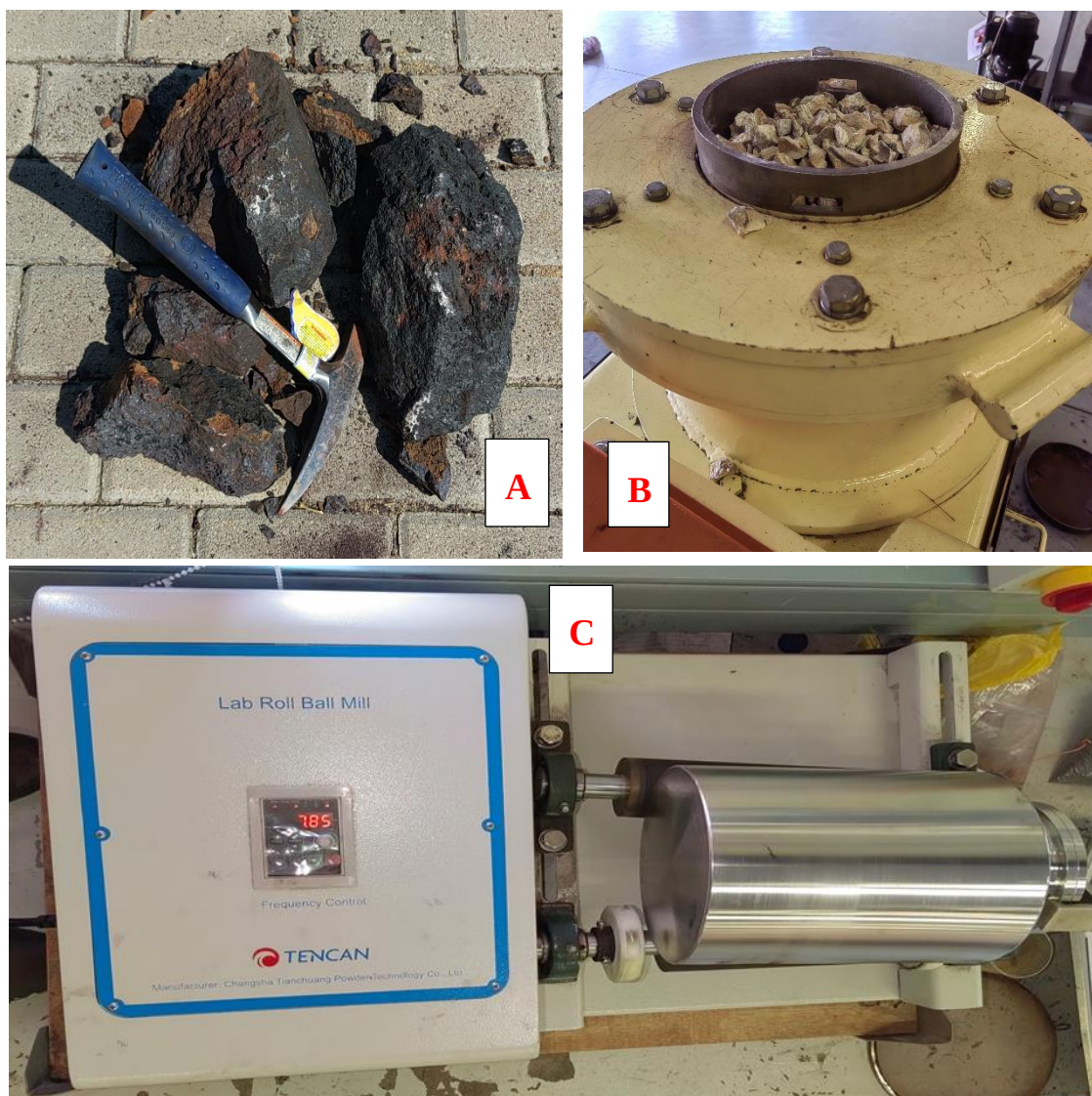
Figure 11. Equipment used in comminution of raw materials; a) Rock pick, b) Cone crusher, c) Ball mill
