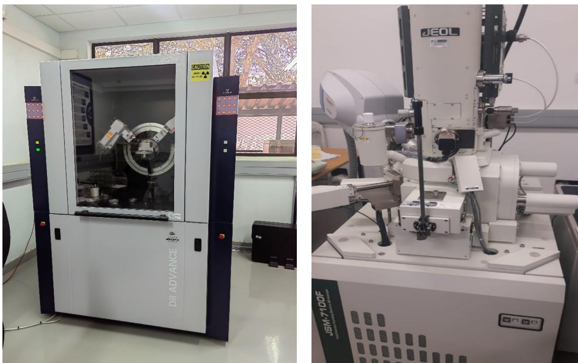
Figure 15. a) D8 Advance Bunker XRD; b) JSM-7100F Scanning Electron Microscope
