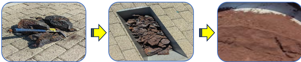
Figure 10. Size reduction from ROM to about 40-120 \mu\text{m}
