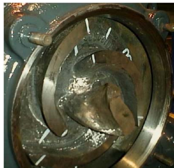
Figure 1.5. Shrouded centrifugal pump impeller (Addie et al. , 2007).
