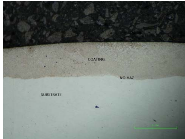
Figure 1.3: A well bonded Tribaloy T800 clad on a 304L stainless steel substrate.
