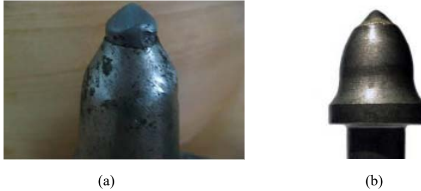
Figure 2.10: Worn shearer pick (a) and laser cladding repaired shearer pick (b). (Source: Che et al. , 2014).
