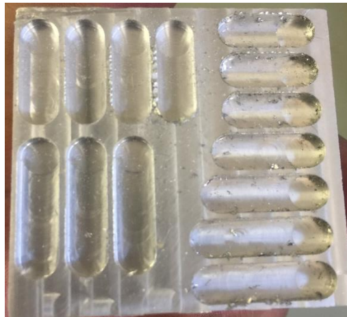
Figure 3. 5: Cuts produce at different feedrates, along the x-axis and y-axis directions
