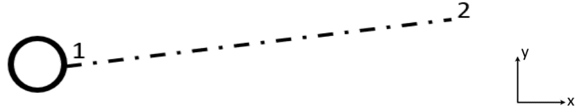
Figure 4. 2: Point 1 represents the starting point of the cutting tool while point 2 represents its end point during rapid motion or linear interpolation.
