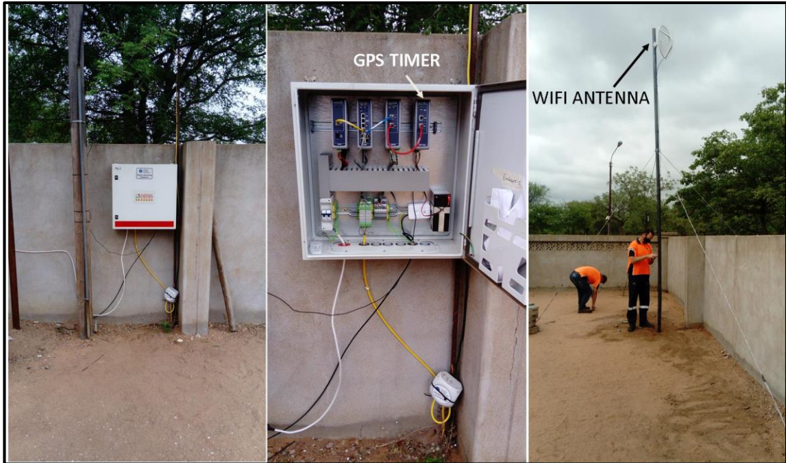
694 Figure 3.7: Surface seismological monitoring equipment setup.
