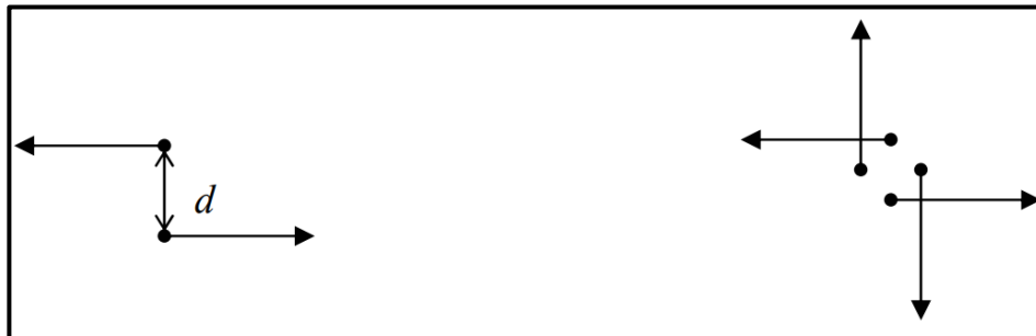
402 403 Figure 2.6: Balanced double-couple (right) and unbalanced force couple (left).
