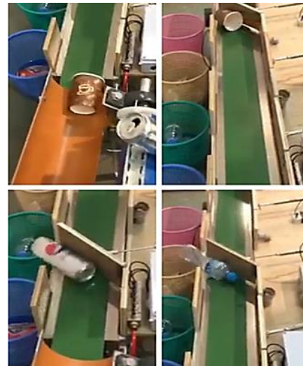
Fig. 7. Sorting process of the solid waste segregation system
