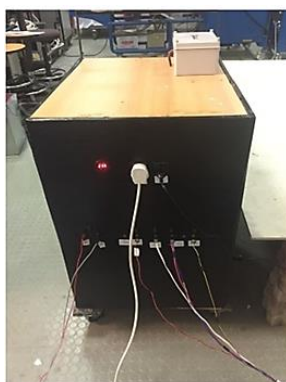
Fig. 10. Solar power conversion system for the solid waste segregator
