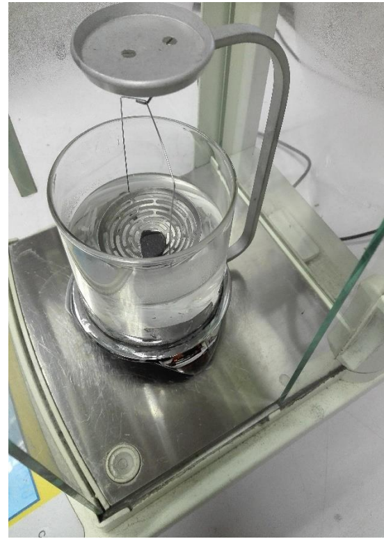
Figure 3.7b: Weighing density of a pellet in water.
