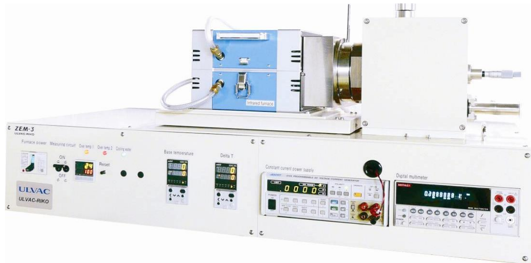
Figure 3.17: A picture of ZEM-3 (Ulvac-Riko) instrument [63].
