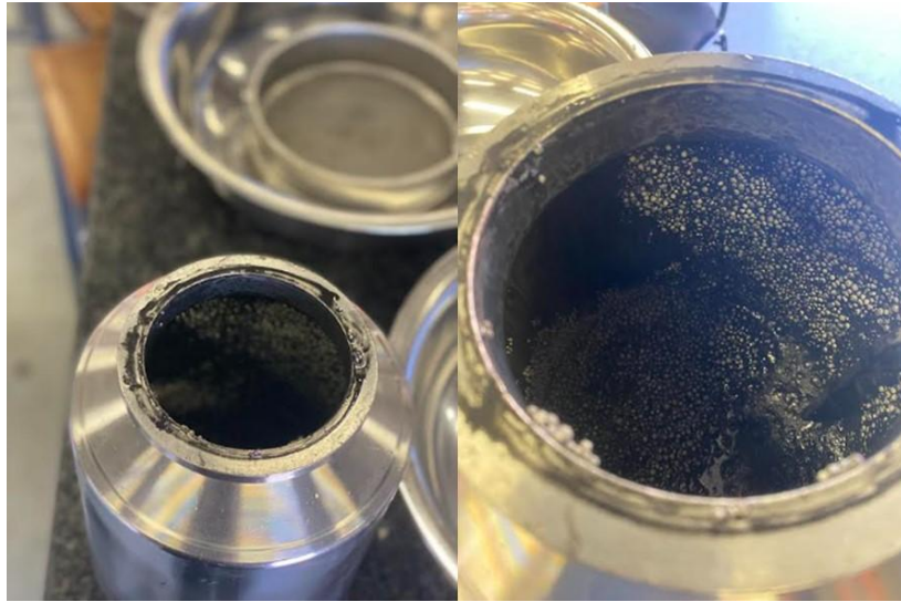
Figure 5-4: Mill contents sticking on internal mill surface, due to the impact of high milling speeds on efficiency of ball mills.
