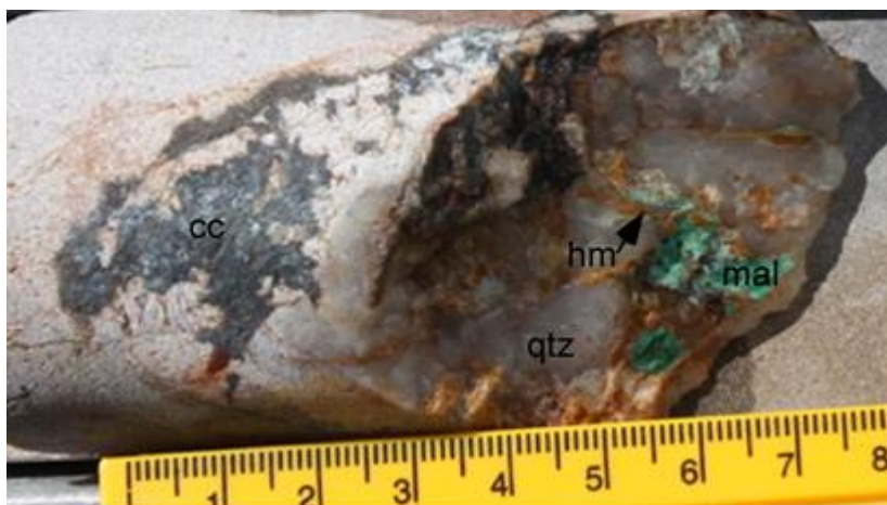
Fig. 6.7. Photograph showing supergene mineralisation in a silicified rock. cc; chalcocite, qtz; quartz, hm; hematite, mal; malachite (drill core HA 487-D; 144.13-144.22 m). Note; the primary texture of the rock is completely destroyed; malachite is not genetically related to the silicification.
