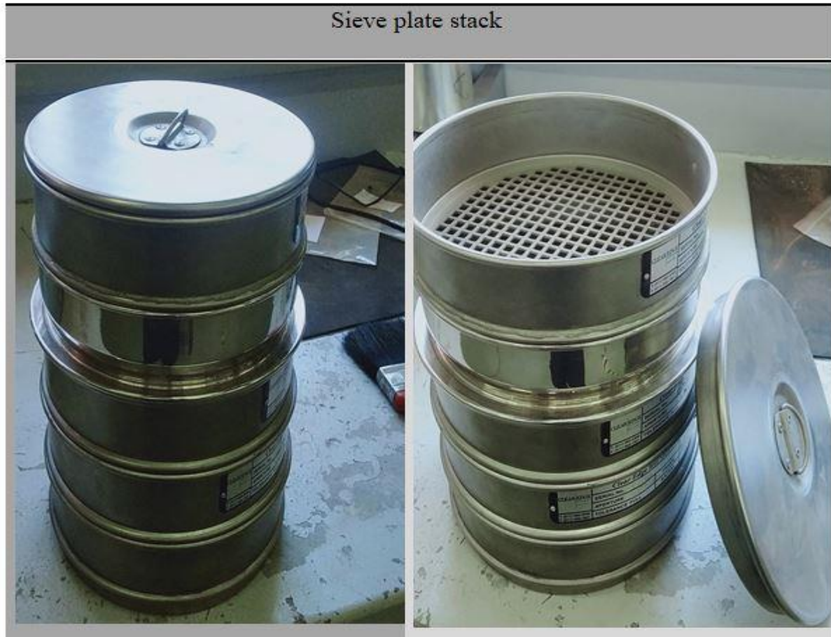
Figure 1.1 showing sieve arrangement stacks that are used for Particle size distribution analysis after a size reduction process (picture taken with a camera)
