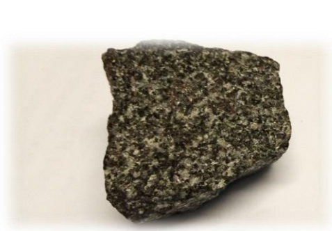
Figure 4.2 Panda quarry diorite rock sample imagery taken with a camera during lab preparation for microstructural imaging
