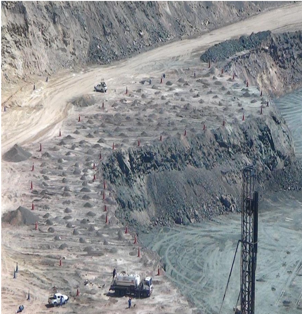
Figure 2. 2. Charged and stemmed blast holes before blasting pattern 845-830IO32-37.
