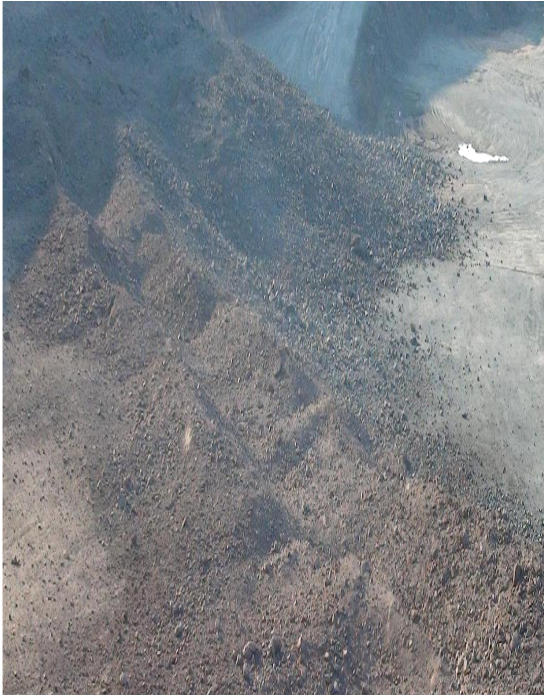
Figure 2. 3. Muck pile distribution after blasting pattern 845-830IO32-37
