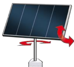
Figure 1: a dual axis solar taking mechanism. Source [10]
