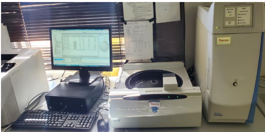
Figure 3.5: Picture showing Dionex Aquion ion chromatography system
