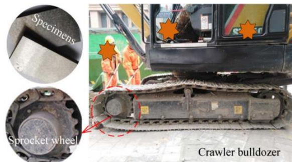
Figure 2.10: Sprocket wheel in contact with crawler Bulldozer chain (Sun et al., 2019; Sobota, 2013)
