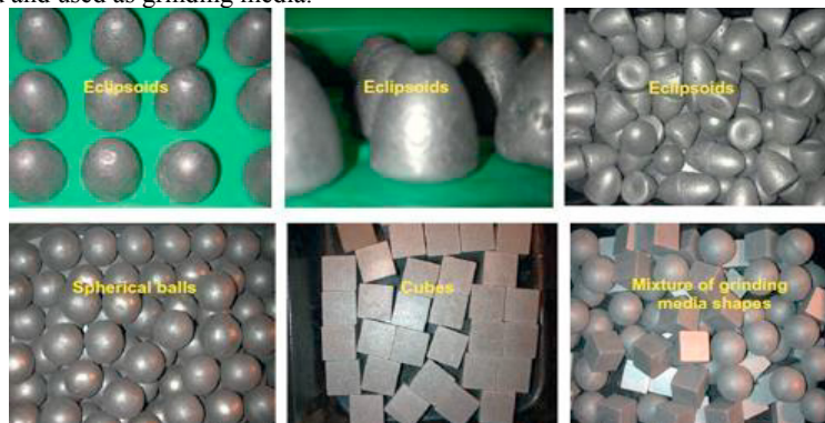
Figure 1: Photographs of cubes, spheres and eclipsoids and mixture of grinding media shapes used for the batch tests [19]
