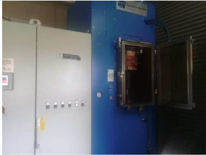
Figure 3-4. FAST/SPS sintering equipment (model FCT Systeme GmbH, Germany)
