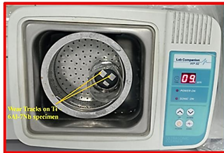
Figure 3. 25: Ultrasonic cleaning of the Ti-6Al-7Nb specimens after wear test prior to SEM analysis of the wear tracks.
