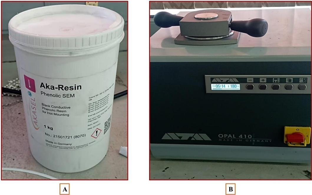
Figure 3. 12: (A) PolyFast resin, a conductive resin used for hot mounting of Ti-6Al-7Nb specimen. (B) An Opal 410 hot mounting press at BIUST’s Materials Laboratory used in this study.
