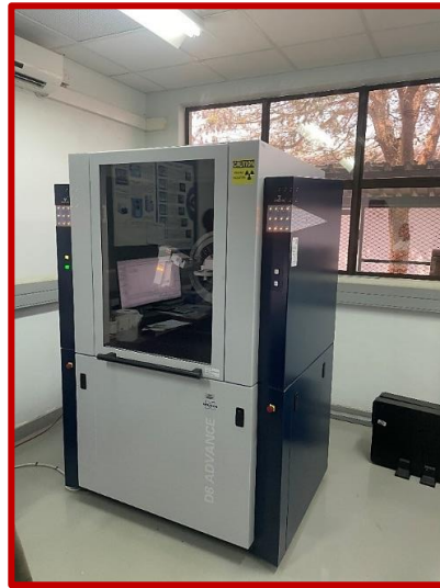
Figure 3. 18: X-ray Diffractometer Bruker D8 Advance utilised in this research at BIUST, Palapye, Botswana.
