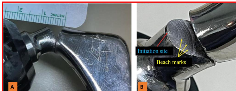
Figure 2. 13: (a) Side view presentation of the failed SS316L femoral implant's neck region. (b) Higher magnification diagonal view displaying the initiation point (red
