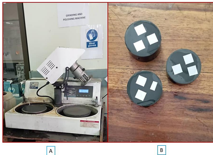
Figure 3. 14: (A) Qualitest Qualipol VTD SA grinding and polishing machine at the BIUST Materials Testing Laboratory. (B) Ground Ti-6Al-7Nb specimens.
