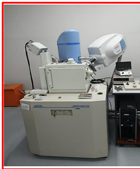
Figure 3. 17: JEOL JSM – 6610 Scanning Electron Microscope used in this study.
