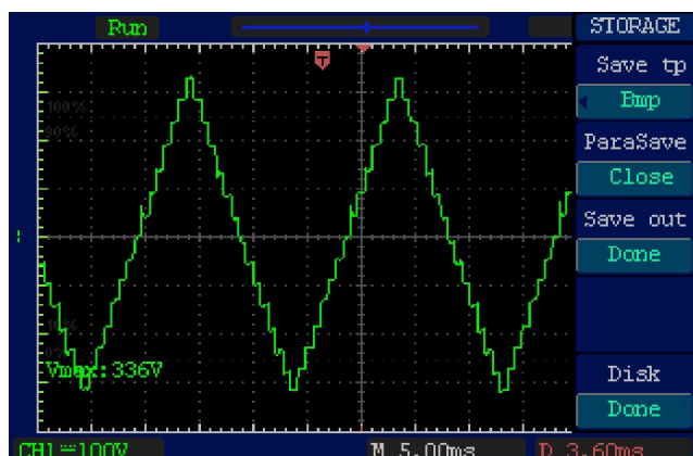
FIGURE 17. Regulated output waveform for voltage in open loop condition.
