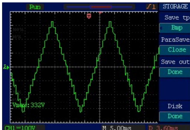
FIGURE 18. Regulated output waveform for voltage in closed loop condition.
