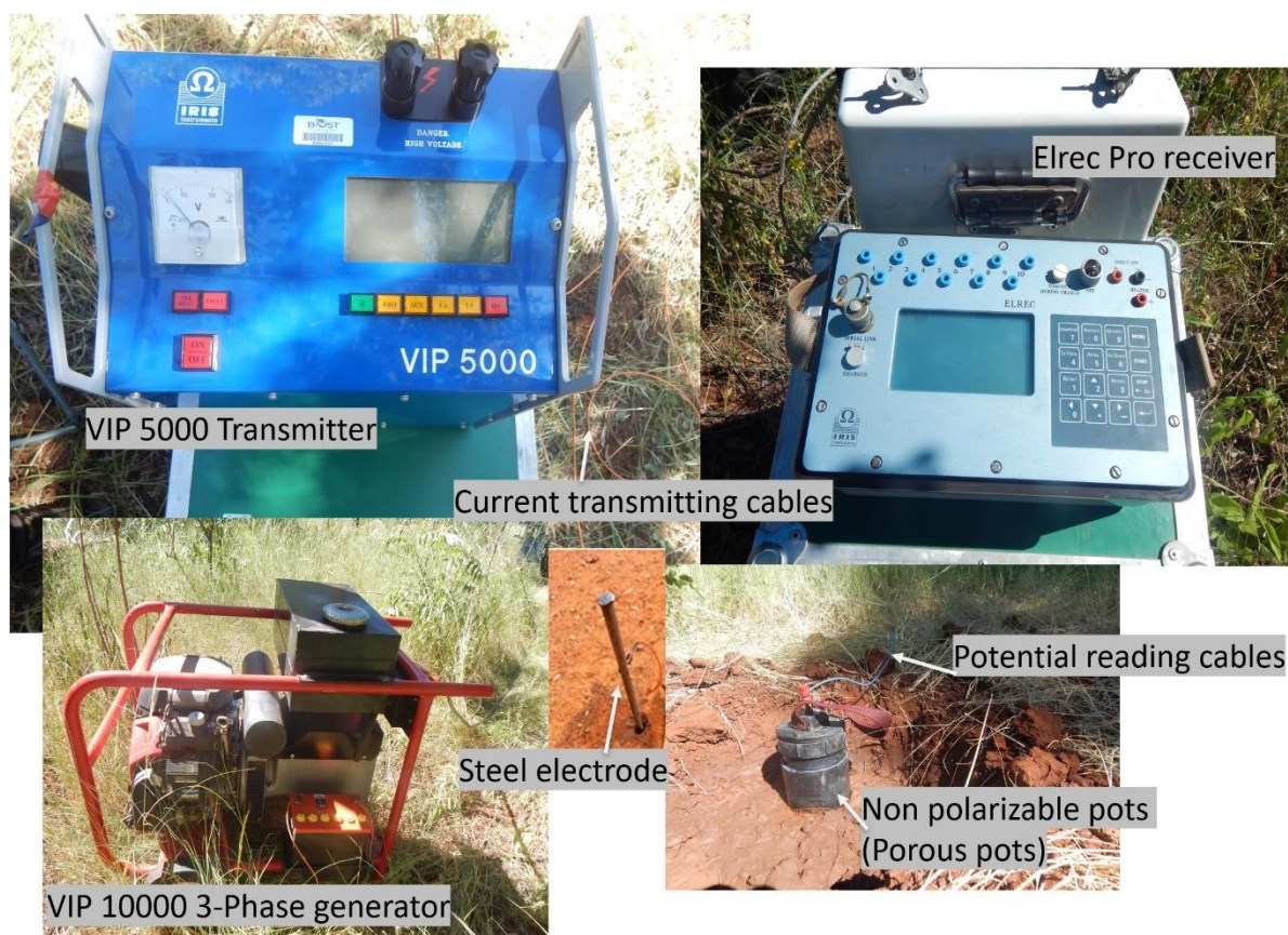
Figure 5.1: IP-ERI geophysical equipment employed in the survey.
