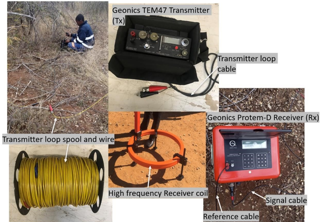
Figure 5.3: TEM data acquisition equipment employed in the survey
