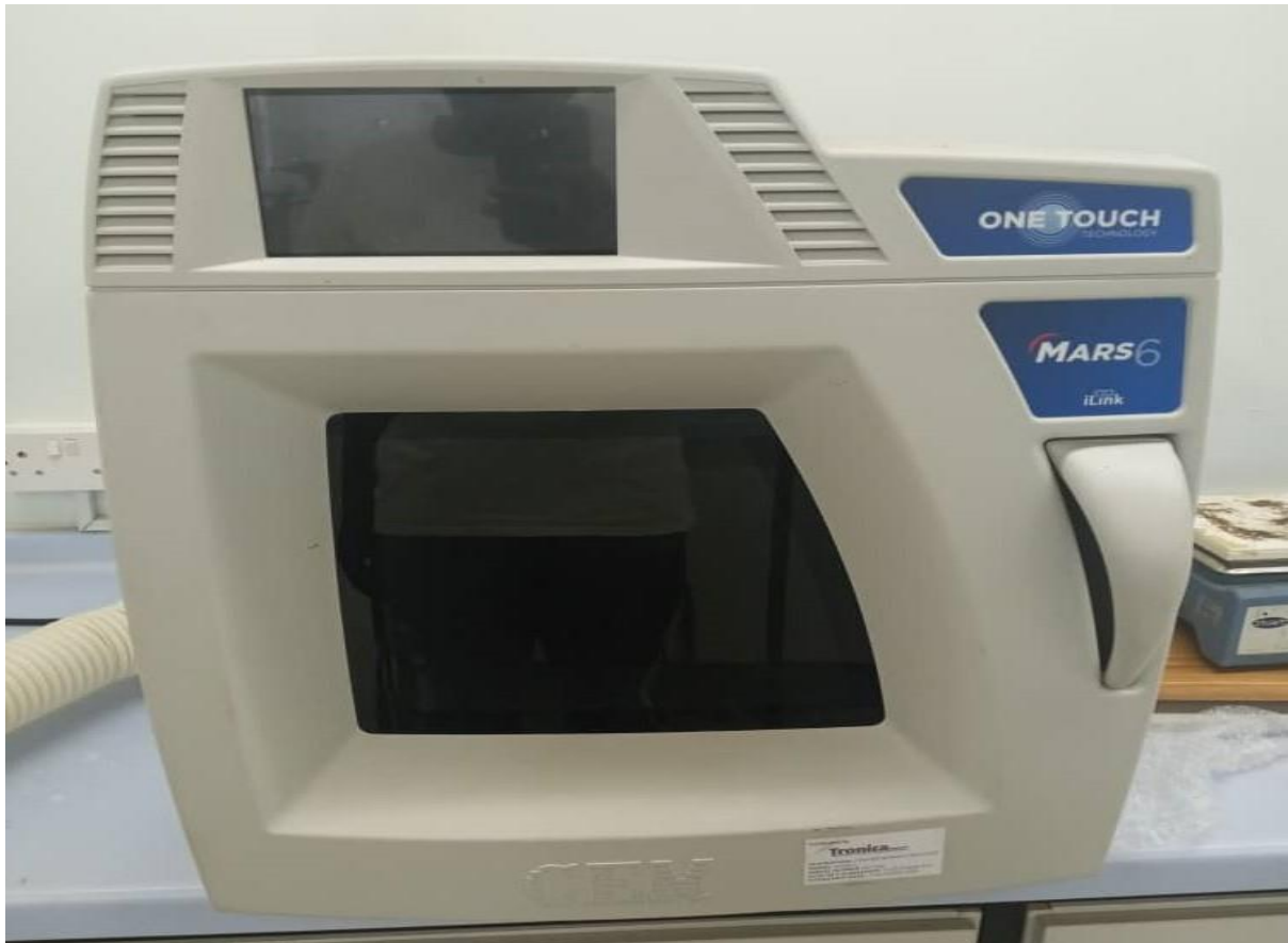
Figure 10. A picture of the BIUST microwave digester used for extraction of heavy metals
