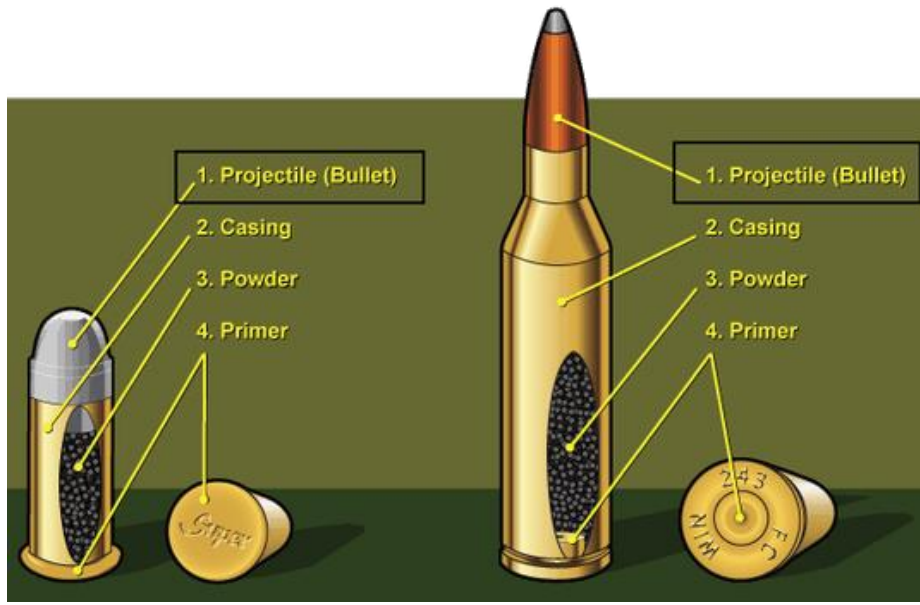
Figure 2: Structure of a Bullet 21
