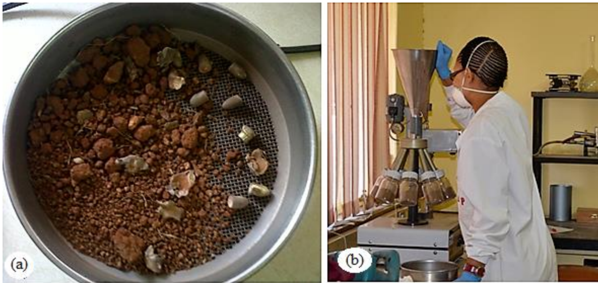
Figure 11: Visibly corroded bullets were witnessed upon sieving with a 2 mm sieve (a) and the electric rotary splitter was used for homogenising the soil samples as shown in (b) above.
