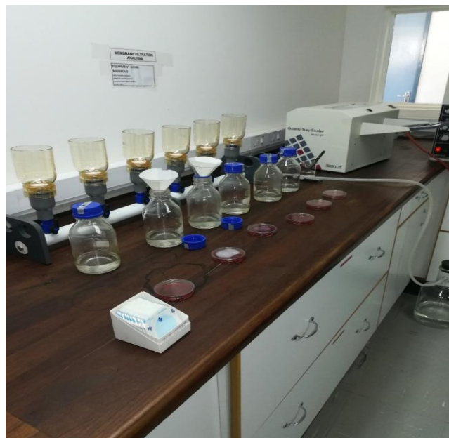
Fig. 1; Membrane Filtration Analysis equipment used for analysing the effect of MO extract on Total coliform bacteria
