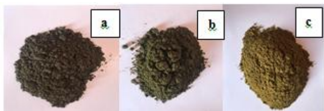
Fig.2: Fly Ash based coagulants (a) raw fly ash (b) calcined fly ash (c) calcined fly ash-sodium hydroxide complex
