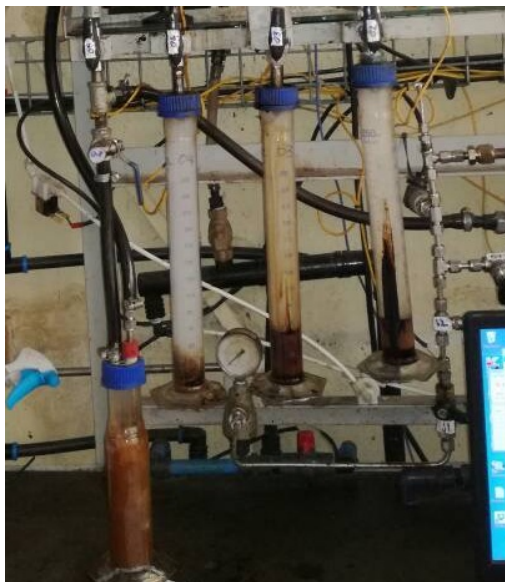
Fig. 3. liquids products, from right to left; heavy oils, light oils, clear liquid. On the counter is a bubbler
