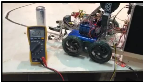
Fig 10. Robot parks in the docking bay for wireless charging operation
