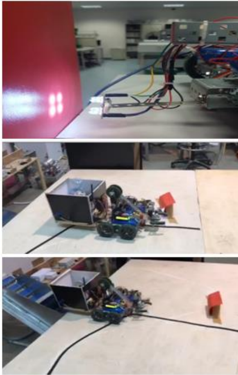
Fig. 9. Color sensing operation of the trash collector robot
