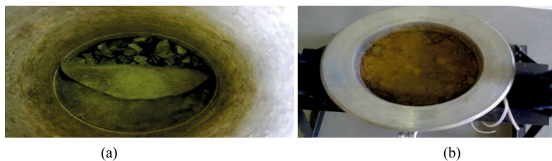
Fig. 5. (a) Hydrated geotextile on porous stone to prevent outlet clogging; (b) Lightly rammed AS to simulate loosed subsoil
