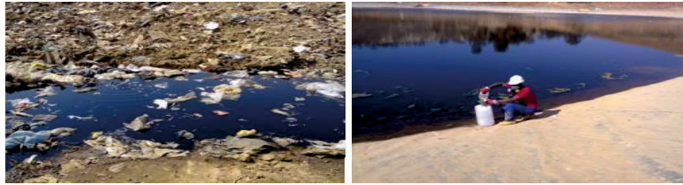
Fig. 3. Permeant/ leachate sampling from leachate pond in-situ
