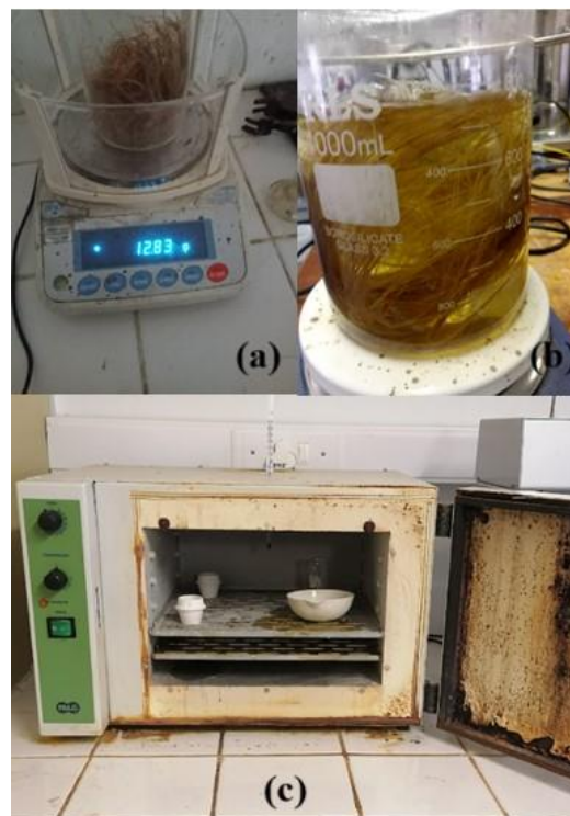
Figure 3.8: (a) Fibre weighing (b) Boiling test (c) Oven-drying.
