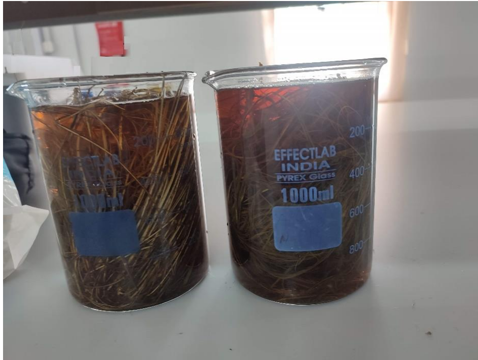
Figure 3.3: Alkali treatment of Mokolwane Fibres
