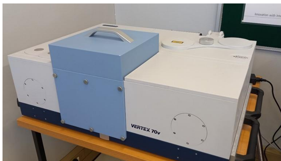
Figure 3.10: Bruker Vertex 70V vacuum FT-IR spectrometer
