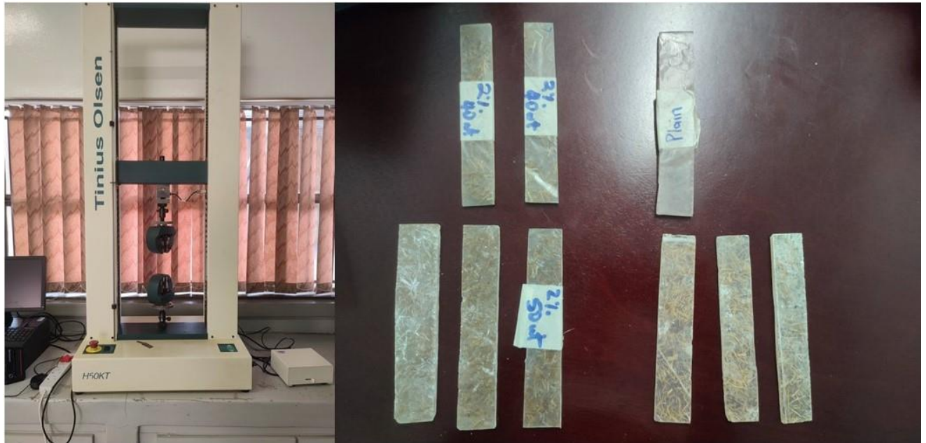
Figure 3.15: (a) Tinius Olsen H50KT Universal Testing Machine (b) Tensile test samples
