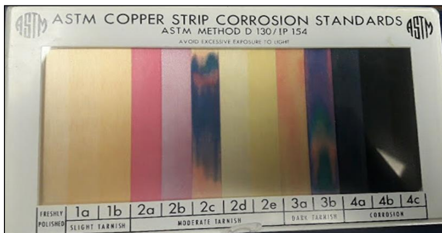
Figure 7. Copper strip corrosion levels of ASTM copper strip corrosion standards
