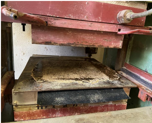
9 Figure 3-10: (a) Composite board after pressing (b) Cooling and compression of composite board.
