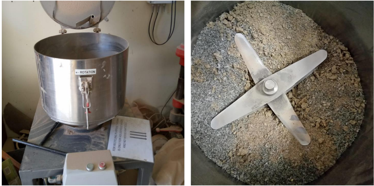
2 Figure 3-8: (a) Compounding machine (b) Fiber particles and LDPE granules inside machine
