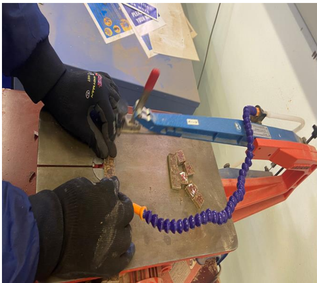
12 Figure 3-13: (a) Cutting boards into sample sizes (b) Boards stacked for conditioning.
