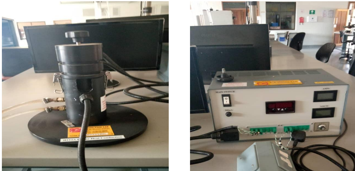
Figure 3-17: Linear heat conduction unit H112A
