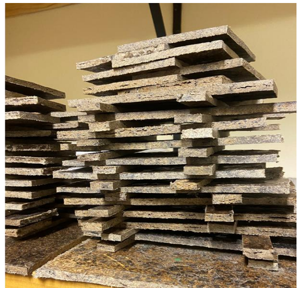
12 Figure 3-13: (a) Cutting boards into sample sizes (b) Boards stacked for conditioning.
