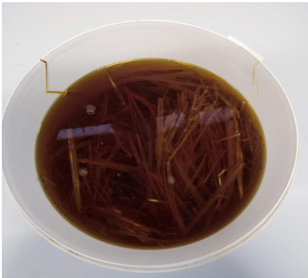
2 Figure 3-3: Water Retting of sorghum stalks
