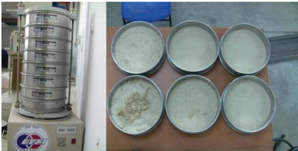
8 Figure 3-7: The round vibratory sieves (b) the sieves with Sorghum AR particle fiber
