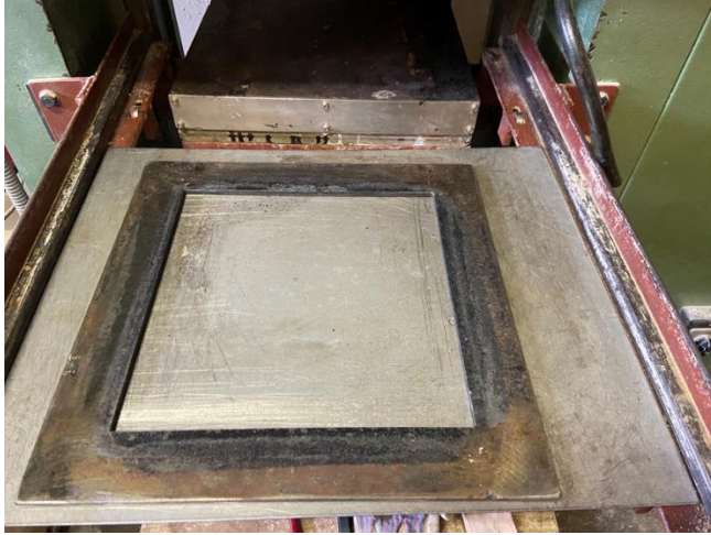
2 Figure 3-9: (a) Compression moulding mould (b) Removal of extra moisture
