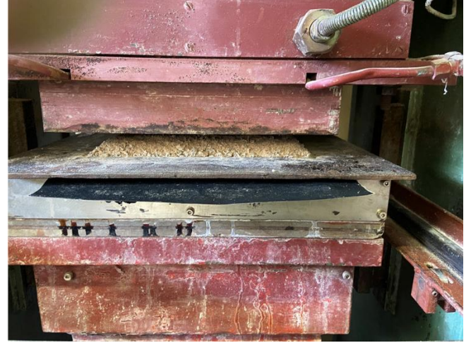
2 Figure 3-9: (a) Compression moulding mould (b) Removal of extra moisture
