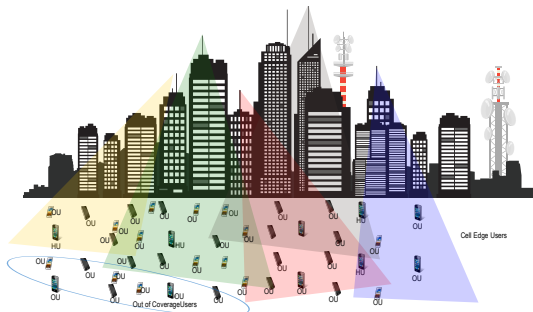
FIGURE 4.1: Distribution of users over a heterogeneous network under the assumption that OUs are cell edge users.
