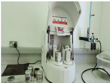
Figure 4. Showing a planetary ball mill for grinding and pulverizing samples depending on device settings. Picture was taken during laboratory experimentation.
