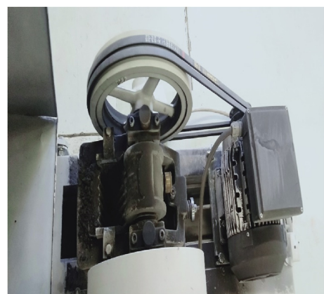
Figure 2. Shows a pictorial laboratory double-toggle Jaw crusher equipment with 100 mm × 150 mm gape opening and 190 depth of crushing chamber.
