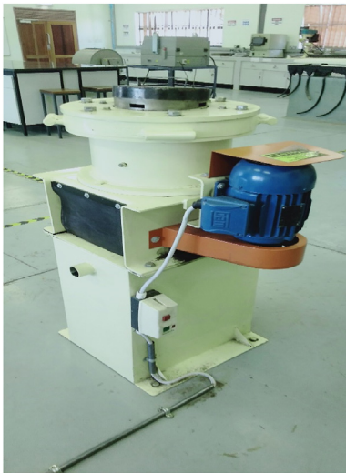
Figure 3. Showing the pictorial image of the laboratory gyrotory crusher used for secondary crushing.
