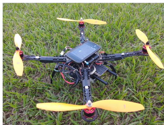
Fig. 9 Quadcopter used in [101] with an on-board smartphone as flight controller. Picture reprinted from [101]
