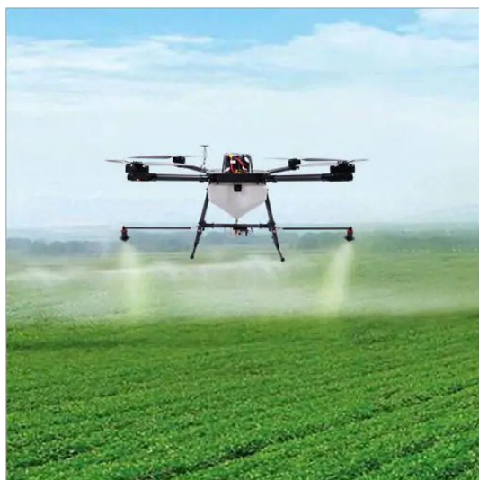
Fig. 2 Quadrotor drone spraying pesticide on crops. Picture reprinted from https://www.indiamart.com
