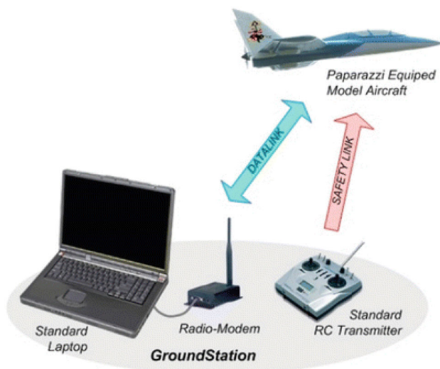
Fig. 10 Platform for drone control from GCS . Picture reprinted from https://www.google.com/search?q=multirotor+UAV++ground+control+station+images
