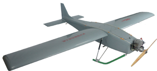
Fig. 1 The KC2800 is a fixed-wing drone used for surveillance and mapping. Picture reprinted from https://aibirduav.diytrade.com
