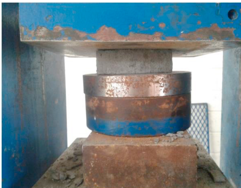
Fig. 3. Brick compression tests
