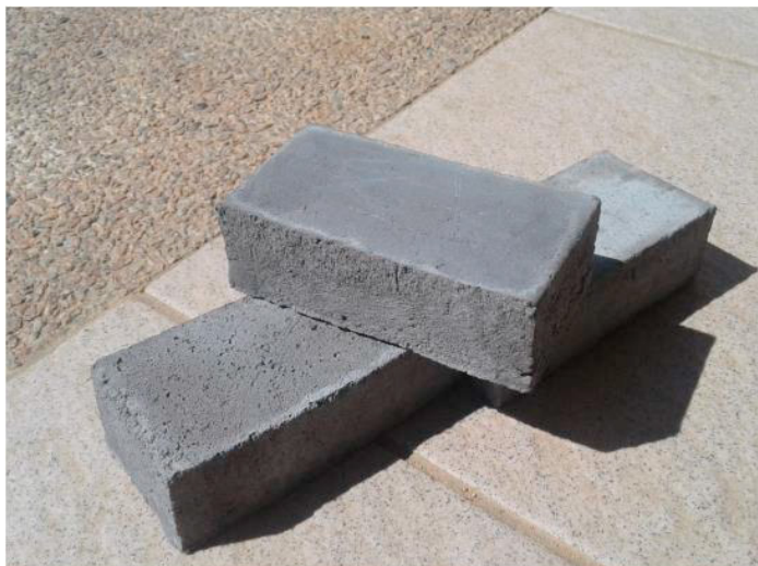
Fig. 4. Sodium silicate treated coal ash brick
