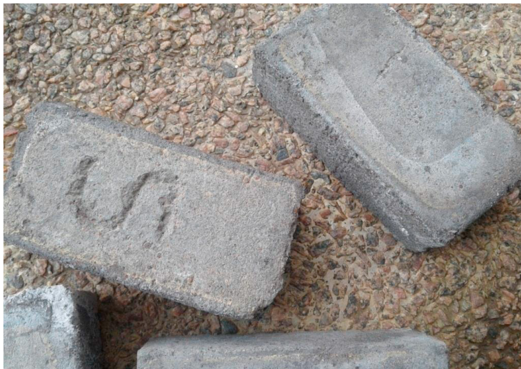
Fig. 7. Appearance of bricks with low sodium silicate content after exposure to ammonium nitrate
